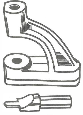
Use this tool for drilling and countersinking lining.
