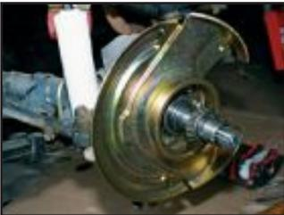
2). Next, place the rotor behind the hub and have the wheel studs pressed through the rotor and into the hub. If you don't put the rotor behind the hub, your brakes won't line up with the calipers.
