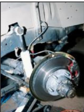
6). Once you have removed enough material, you can then begin rebuilding your front axle. Now would be a good time to replace those worn-out bearings and seals. Remember to pack the bearings and grease everything.
