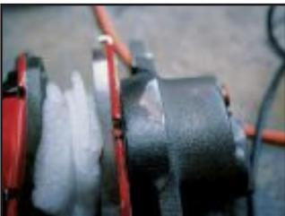
5). Also grind the caliper a little to make sure that there will be no contact between it and the knuckle as the pads wear out, but be careful not to grind through the casting.
