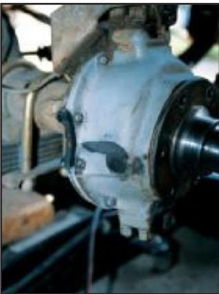
3). Attach the spindle and caliper mounting brackets with a couple bolts to test for caliper fitment. You will need to replace the 12 (six per side) original fine-thread backing plate bolts with ones that are 1-inch long.
