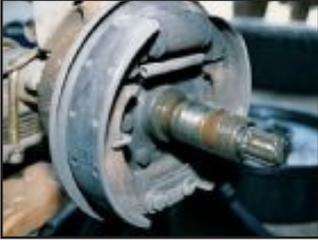
1). Start out by stripping off all of your old drum brake stuff. That's right: down to the spindle. Now that you have the hub and drum off, press the old wheel studs out.
