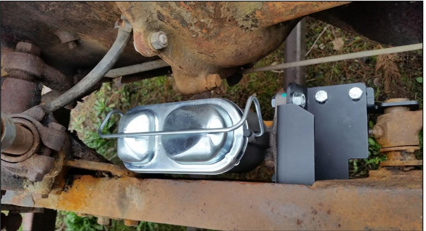
***This is what the kit installed looks like from the top (no body on this Jeep) in relationship to the clutch tube cross shaft, but it also leaves room for adjustment in whichever direction.***
