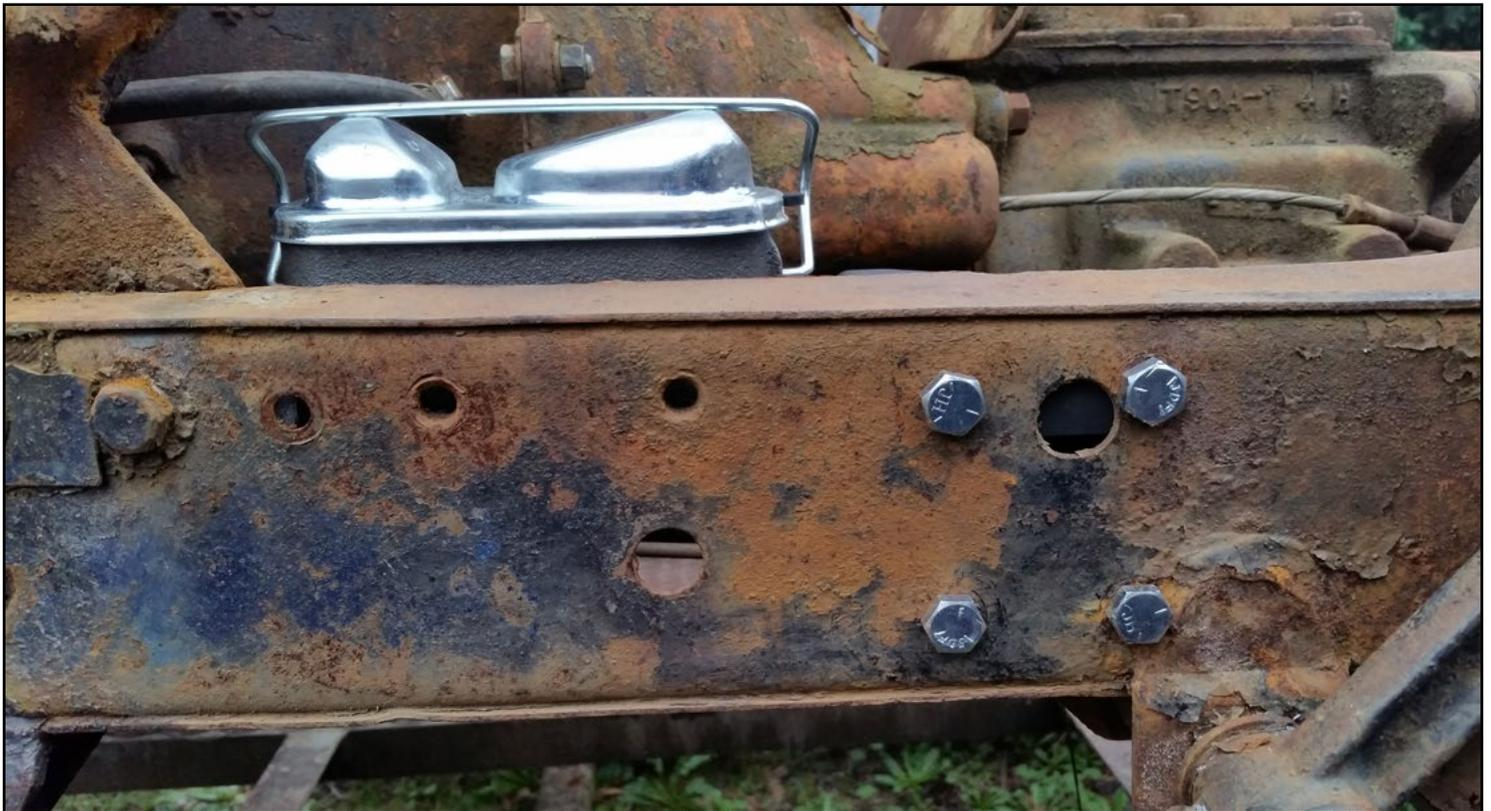
***The location to drill the holes depends on the model and year of your Jeep, and even if there is an existing hole interfering with where you need to drill, flat washers can be used to compensate.***
