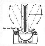
**ROPE SEALS:** Install the seals into the grooves of the cap and block by firmly pressing the packing into the grooves using a "packing tool".
