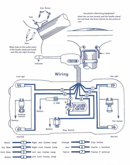
as each cord can be distinguishable by color, the wiring should be man: according to the above drawing \* Notice: Cam is not eed to install for non cancelling Switch.
