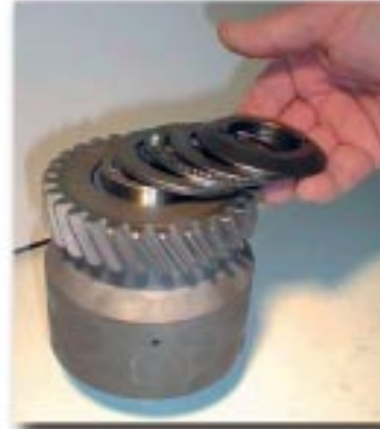
Step P3 Remove the thrust bearing sets. Take note that the thickest race is next to the gear housing.
