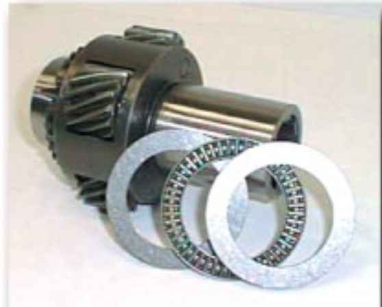
Step P4 Remove the thrust washers & bearing. Take note that the thin race is next to the spider assembly.
