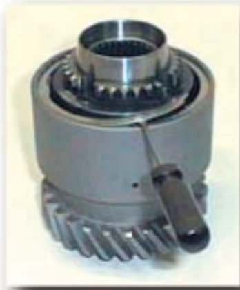
Step P1 Using a small flathead screwdriver, remove the snap ring from the gear housing.
